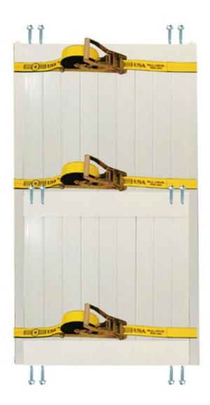
Strap the gate together and pull the rails snug against the uprights. Measure from the edge of rail on each side 1" and 3" and apply the self tapping screws in the top rail, bottom of bottom rail and middle of mid rail. Place the screw caps on the top and mid rail screws.
